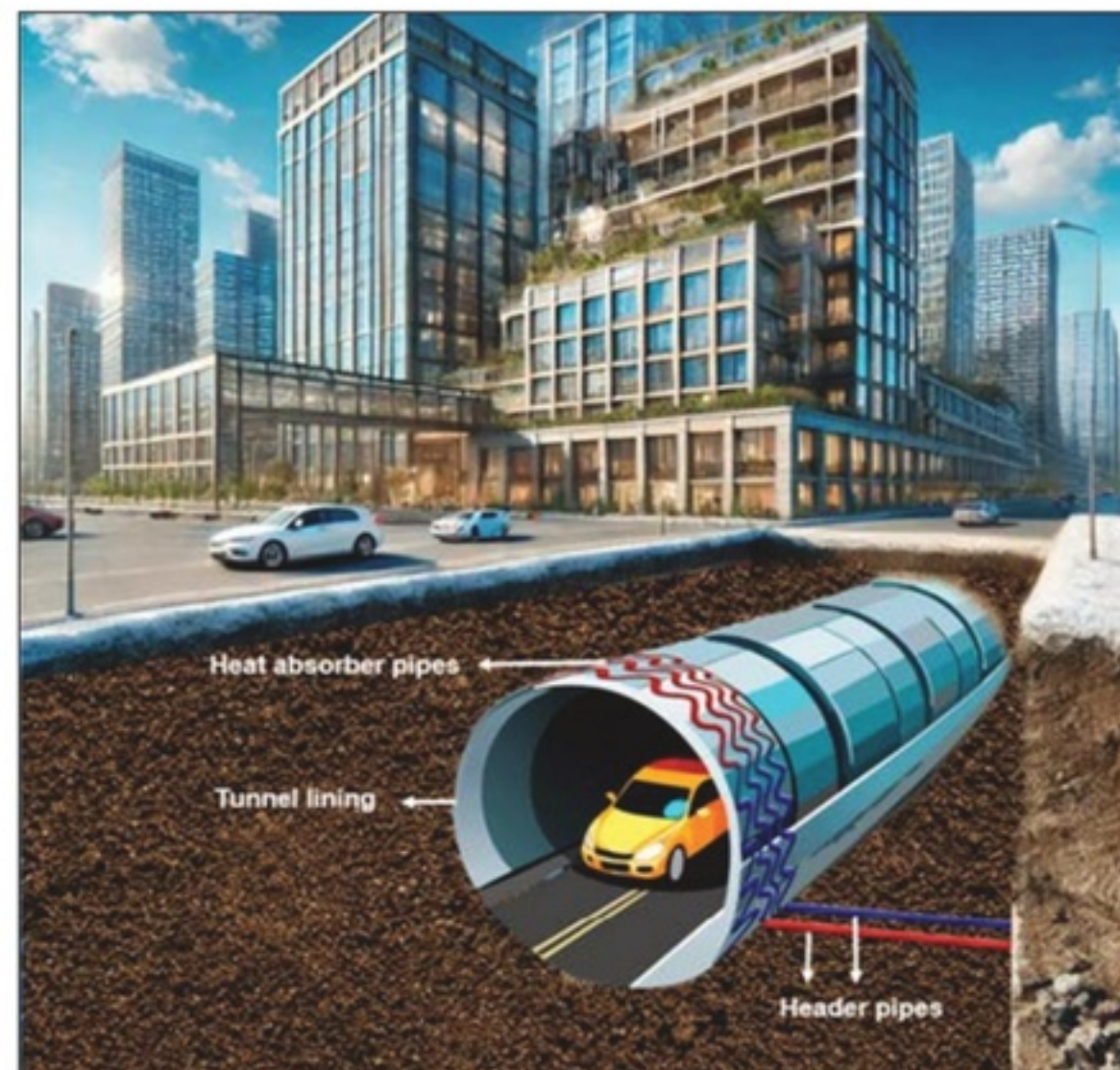
Figure 3- Schematic of an energy tunnel providing space heating and cooling to a building (not to scale).
