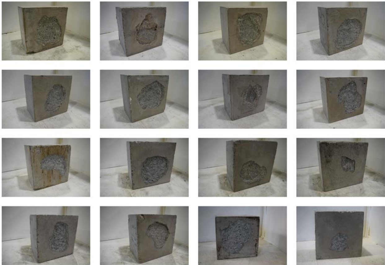
Fig. 6. Photograph for each sample spalled.
