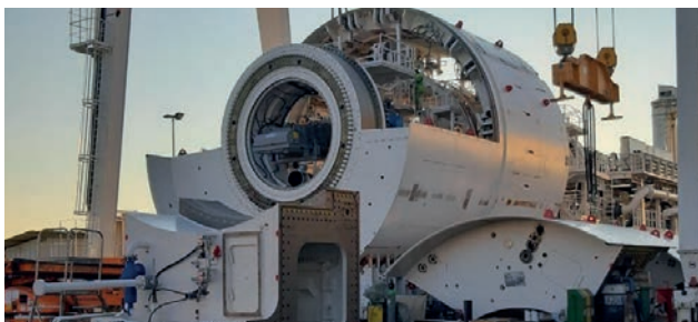
The Herrenknecht TBM that will connect Tantangara Reservoir to the new Snowy 2.0 underground power station.
