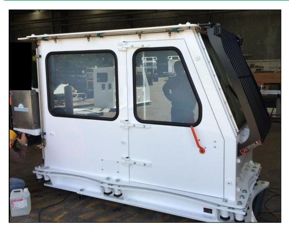
Figure 2: Custom-built roadheader cabin with filters located on the Left Hand Side (rear of cabin)
