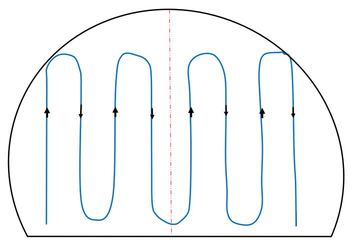
Figure 7 – Traversing pattern for ventilation surveys: Cross section of the tunnel
