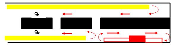
When jet fans are used in the two tubes which are not segregated, the imbalance in thrust creates a recirculation circuit. This is evident by high velocities in localised areas where there is a jet fan nearby. Recirculation can be effectively used in certain occasions to increase the personnel comfort. Care must be given in all instances to avoid build-up of toxic atmospheres.
