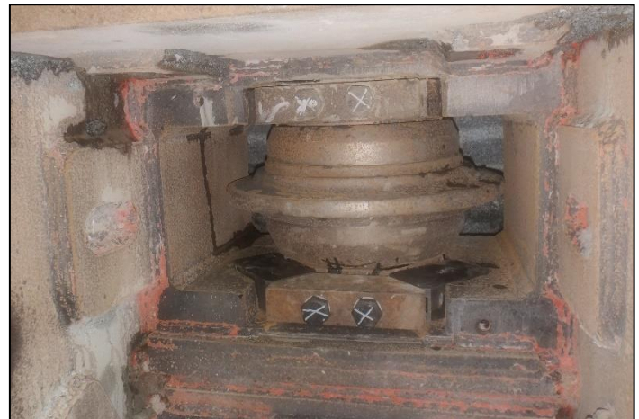
Figure 9: Double wedge block system was used to secure the 19inch disc cutters in the housing
