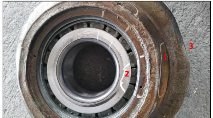
Figure 11: Damaged or worn hubs (1) can cause bearings to either seize or crack (2), resulting in flatspotting of the retaining ring (3)
