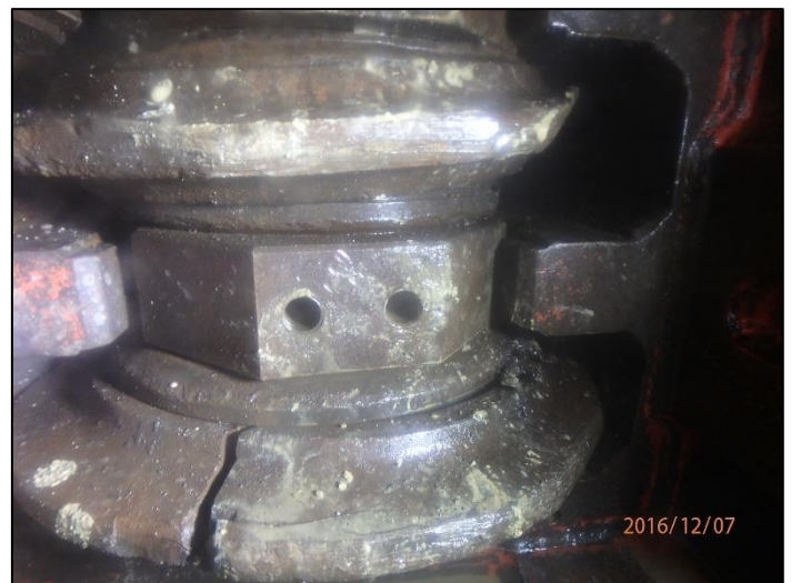
Figure 12: Loose and fallen wedges can further damage disc cutters
