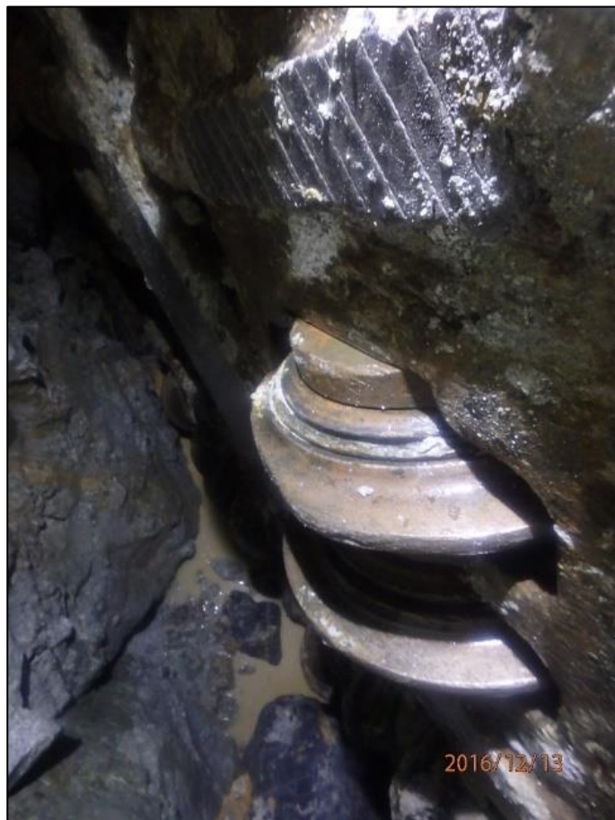
Figure 13: Flatspotting of a double disc cutter in the mixed ground. Note the exposed hub, which is prone to damage and wear
