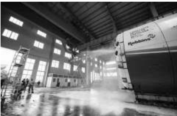
Each Robbins EPB was designed for difficult ground conditions, with a mixed ground cutterhead and newly designed foam and grouting systems.
