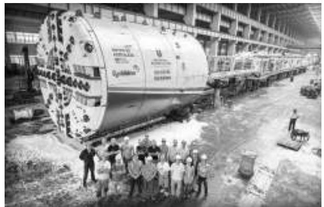
The Robbins crew celebrates the successful testing of the first Metro Fortaleza machine in the company's new Pudong, China factory, seen here after the foam test.
