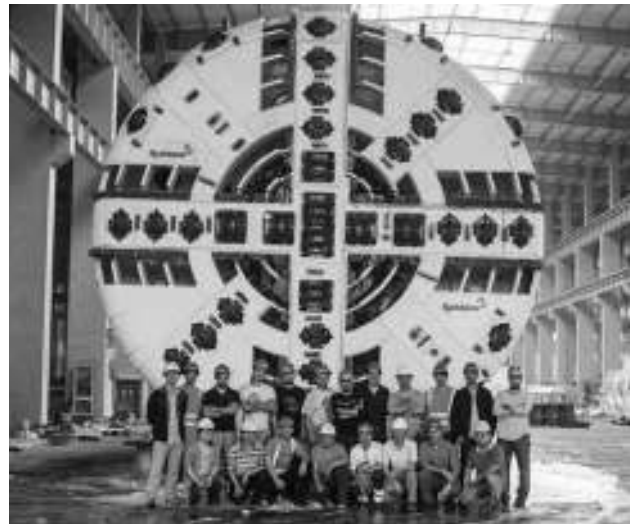
Mixed ground cutterheads on the Robbins EPBs are designed to excavate through abrasive basalt and silty sand under water pressures up to 2.5 bar.
