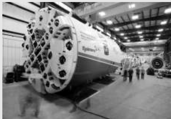
Three new Robbins EPBs and one refurbished machine were custom designed for Moscow's mixed ground ranging from fine sand to stiff clays and boulders.
