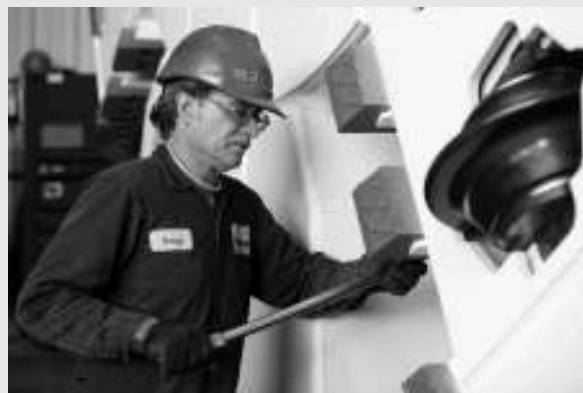
Cutterheads for the Robbins machines have been fitted with interchangeable carbide bits and 17-inch disc cutters.
