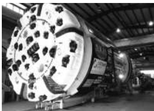
A Robbins Main Beam TBM is preparing to excavate the Indianapolis DRT for JV contractor Shea/Kiewit. The contractor-owned machine includes a cutterhead refurbished by Robbins, with 19 inch disc cutters.
