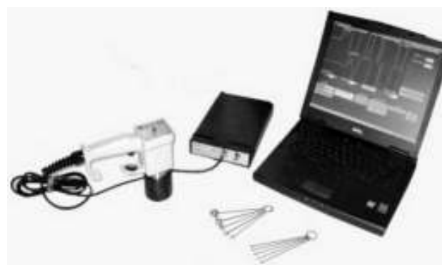
Figure 5 Impact Echo Device (adopted from [16]).
