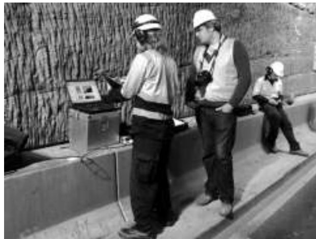
Vibration monitoring equipment in the Norfolk Tunnel 30 April 2011
