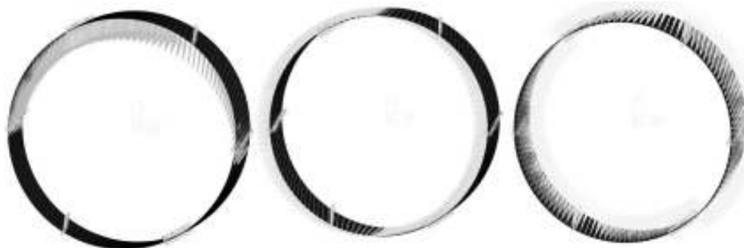
Figure 5: Applied loading in 3D model (a) Vertical rock loading (b) Lateral pressure (c) Hydrostatic loading.
