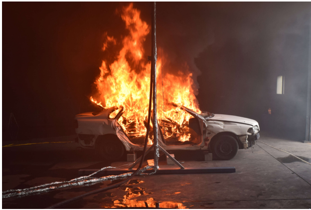
Figure 6: Typical car fire test (prior to activation of the suppression system)
